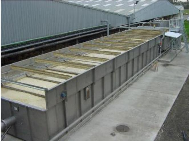
Rendertech Dissolved Air Flotation Plants (DAF) provide the solution to many wastewater treatment problems. They are compact, efficient, simple to operate and economical to run. They can be supplied without chemical treatment, or with chemical treatment to increase the degree of purification.
