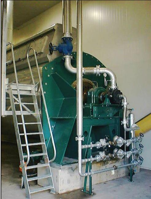
The Rendertech Contact Drier (CD) is an indirect steam heated, continuous drier for drying a variety of granular and fluid products. The construction consists of a horizontal shell with disc rotor for heating and transport of the product.
